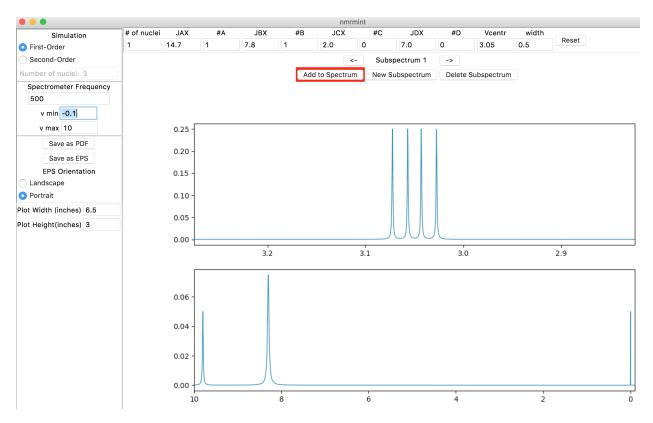
First, we will simulate the ABX system. Click the "New Subspectrum" button in the subspectra navigation panel to create a new subspectrum, then click the "Second-Order" radio button in the upper left "Simulation" panel. The "Number of nuclei" entry below the radio buttons will no longer be greyed out. Enter "3" for the number of nuclei and hit Return/Enter or Tab:
