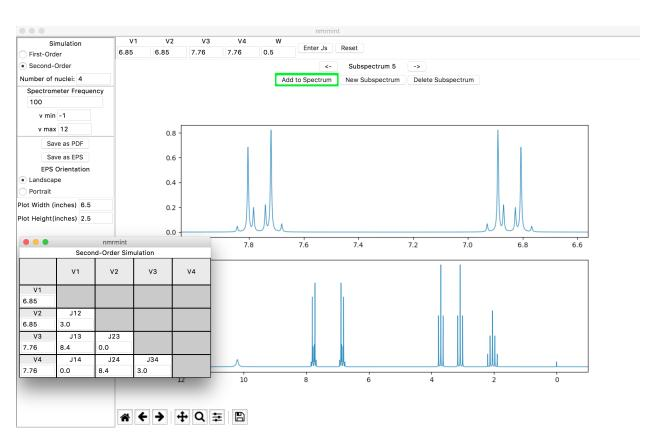
**nmrmint** is an application for creating simulated, complete NMR spectra for use in chemical education. Currently, the application is limited to <sup>1</sup>H NMR only, but expanding this to other nuclei such as <sup>13</sup>C is feasible.
